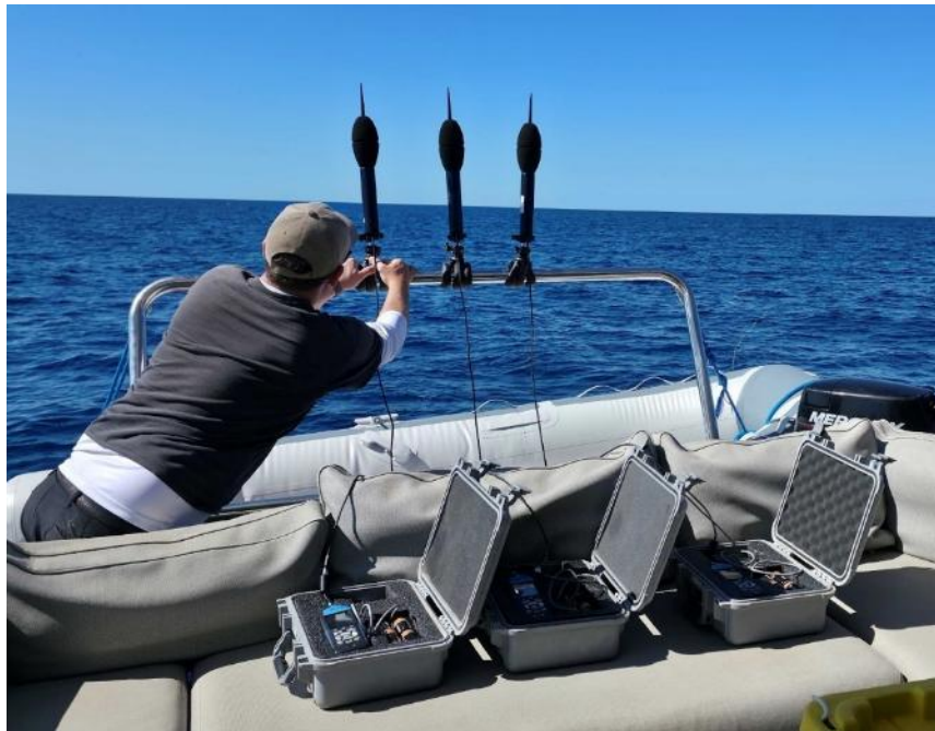
Figure 2-1. Calibration of Larson Davis 831C Sound Level Meters on Monitoring Vessel
